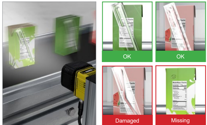
Food & beverage: Identify damaged or missing components
