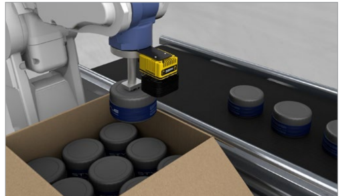
Robotic guidance: Pick and place finished products into bins
