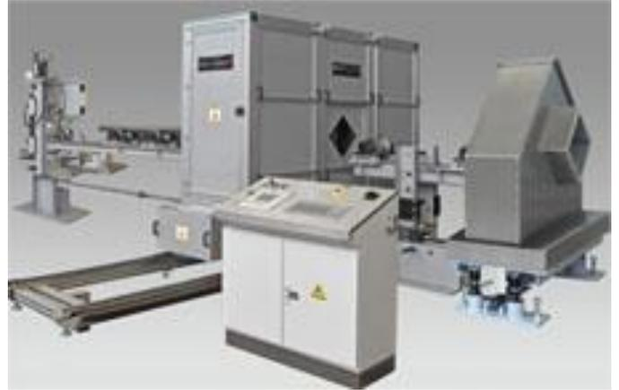
During the casting and rolling mill process of manufacturing steel billets, surface cracks develop. These cracks must be detected and removed before the steel is used.
